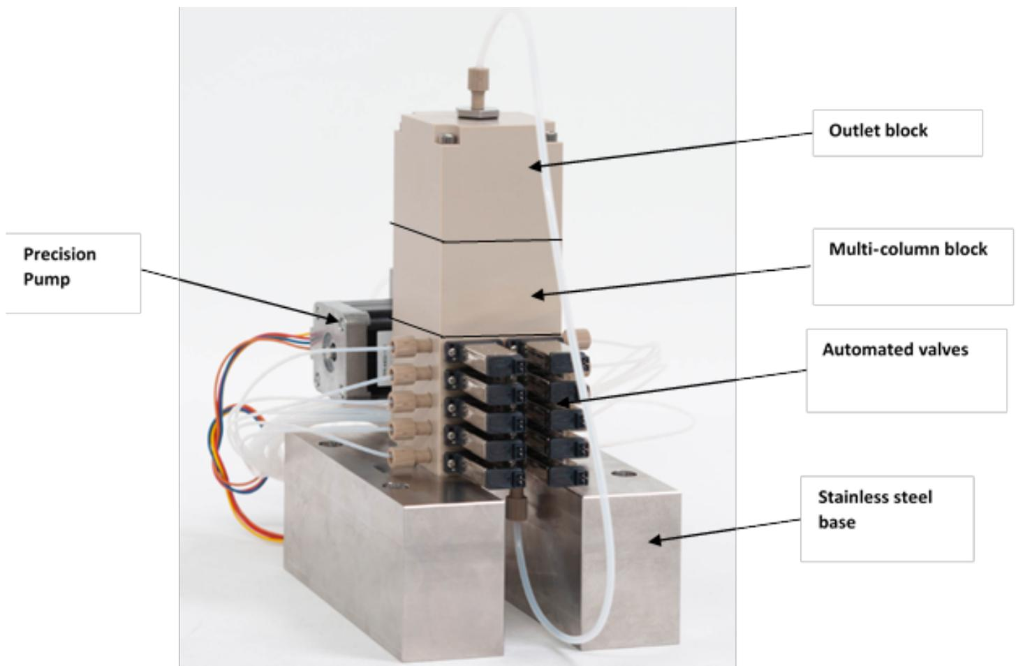
**Figure 1.** XPure-R Rapid Resin Aging System (RRAS)
