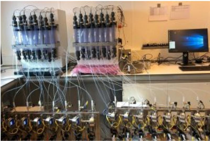
**Figure 1:** Analogy between Symphony orchestra and SMB systems. The XPure automation software on the computer executing the recipe built in the XPure Recipe Manager plays the orchestra maestro's role. a) Orchestra setup playing on musical notes b) XPure SMB system.
