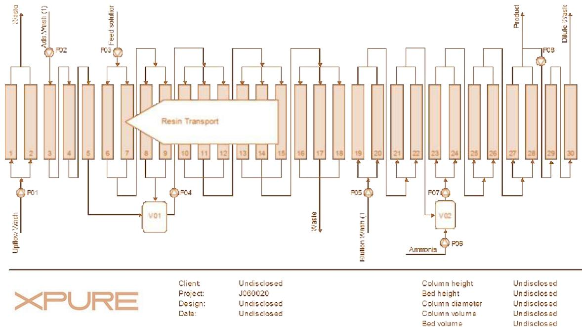
Figure 1. Simplified Process Flow Diagram for the purification of lysine using 30 columns .
