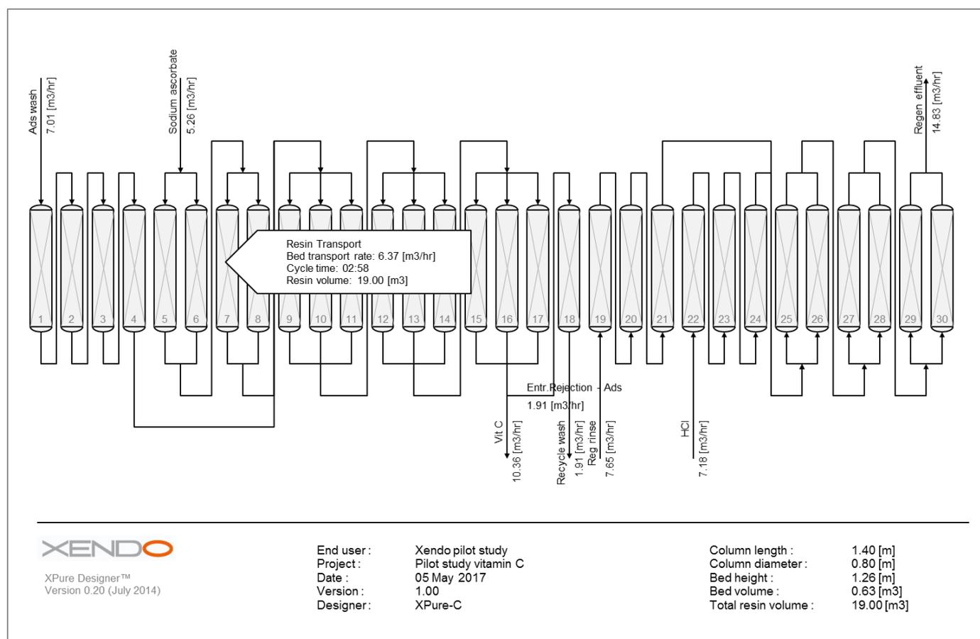
Figure 1. Typical Process Flow Diagram (PDF) for the acidification of sodium ascorbate into ascorbic acid
