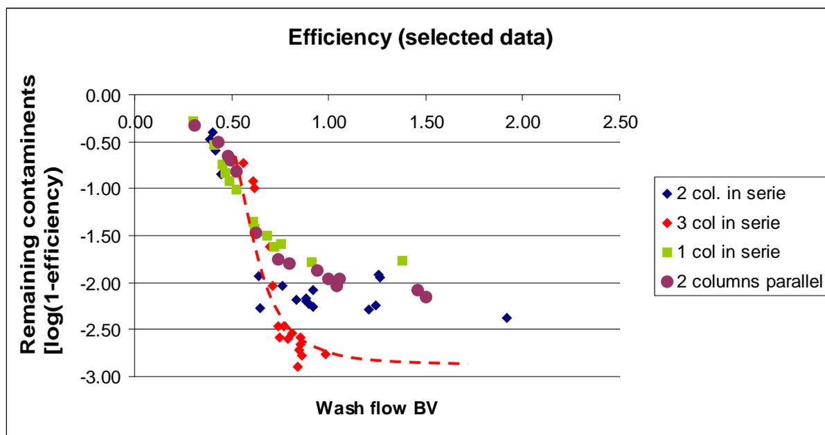
Figure 2: Counter current wash efficiencies in a Carousel unit.<sup>2</sup>
