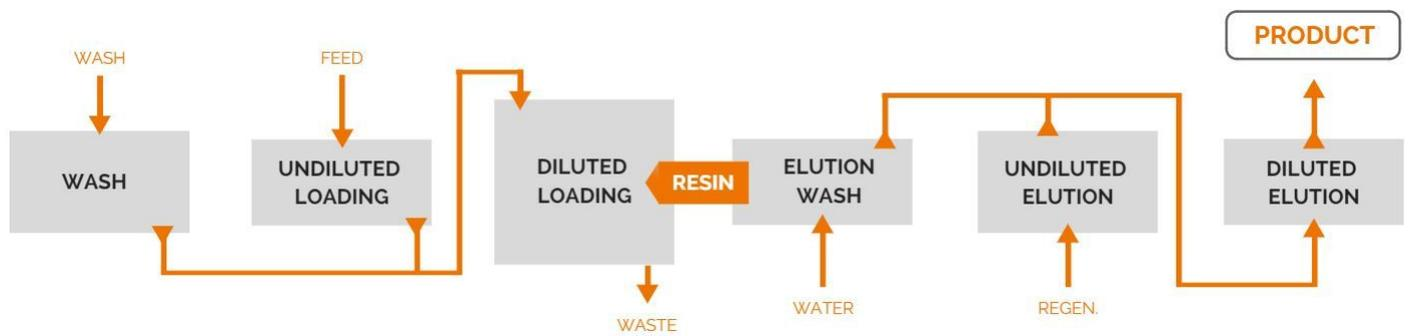
Bind and elute IX chromatography systems based on the SMB principle has opened a huge field of applications where valuable products are recovered or purified on a continuous basis thereby saving substantial water consumption as well as elute and regenerant agent.
