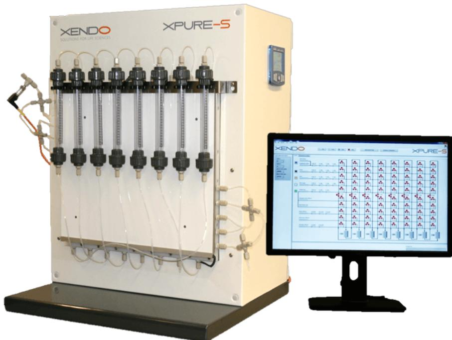
2. A large pilot SMB system featuring a bit larger resin cells from 1-4 inch column diameter on average 400-1000 mm bed height.
