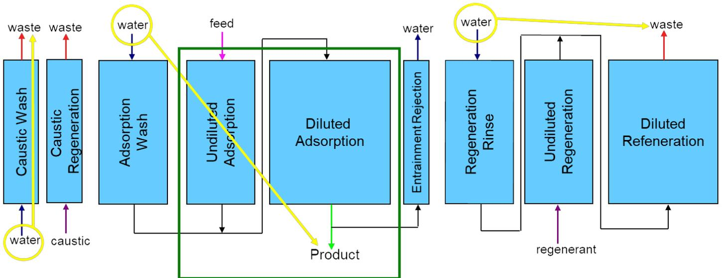
Figure 2. Conceptual design of continuous IX purification for (Product) vitamin C. Each block may contain multiple columns. Total number of columns typically 20-30.
