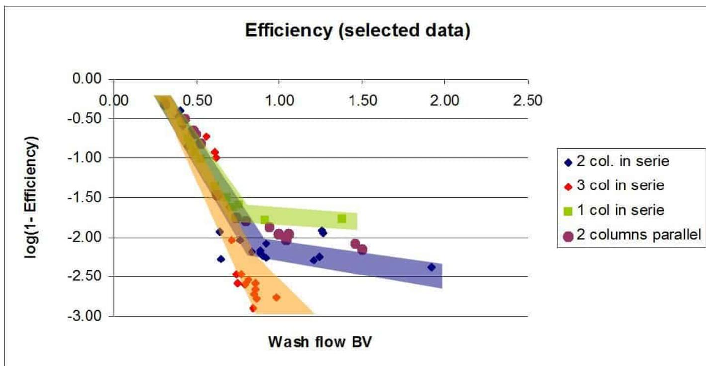
**Figure 3.** Wash efficiency with growing number of counter-current connected columns
