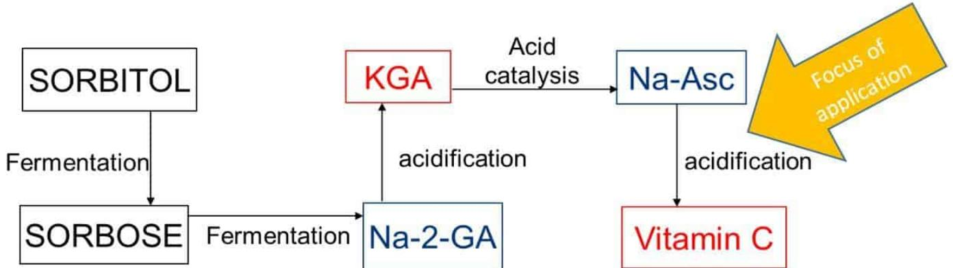
Figure 1. Flow diagram for vitamin C manufacturing
