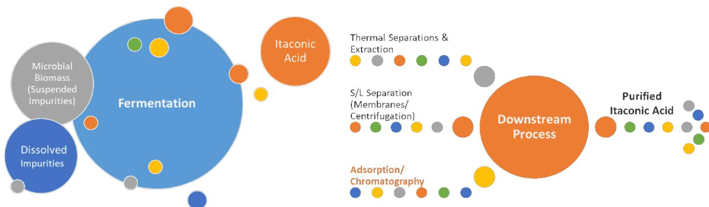
**Figure 1.** Purification of IA requires a downstream process to separate IA from suspended and dissolved impurities
