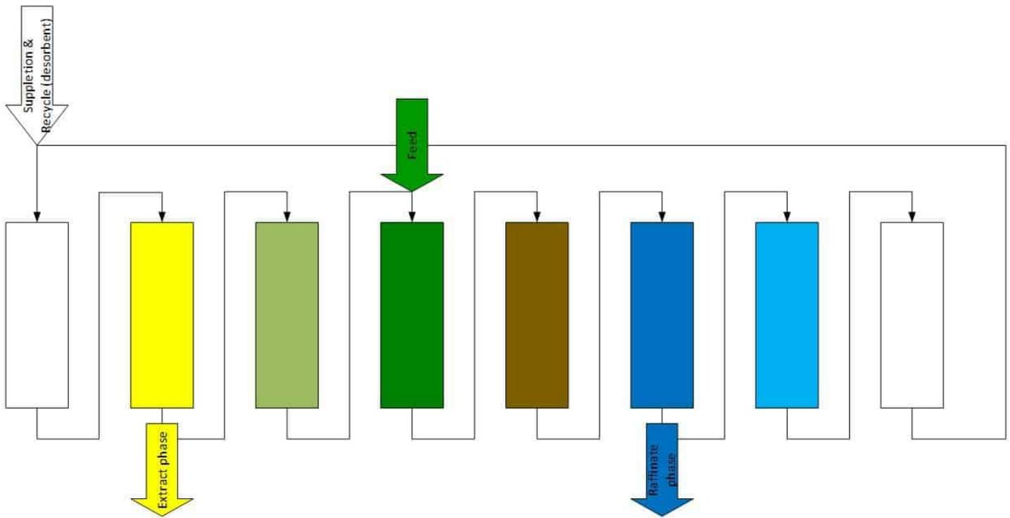
**Figure 3.** Representation of a 4-zone SMB system to separate Fructose (strongest chelating) in Extract Phase (yellow exit) from Glucose (weakest chelating) in Raffinate Phase (blue exit). Green input flow represents the feed mixture. The white influent represents the desorbant buffer, often water.
