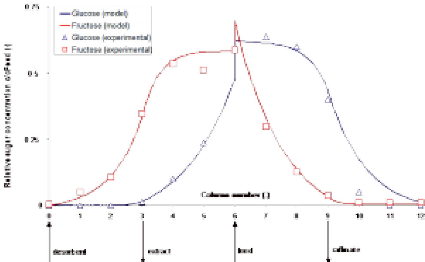
**Figure 2.** Comparison of production data of fructose/glucose fractionation on a 12-column system with calculations according to our process design model
